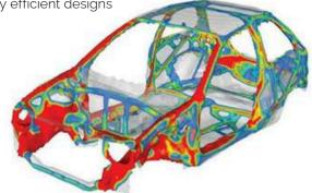
Altair Radioss is a leading structural analysis solver for non-linear problems under dynamic loadings. It is highly differentiated for scalability, quality, robustness, and consists of features for multiphysics simulation and advanced materials such as composites. Altair Radioss is used across many industries worldwide to improve the crashworthiness, safety, and manufacturability of structural designs.
